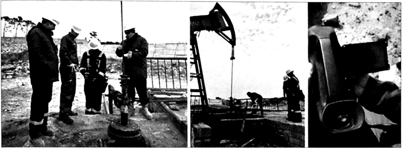
Actual images of the detection & quantification team using the FLIR GFX320 OGI Camera for leak detection (at an oil production wellhead at the Bibiheybatneft OGPD)
